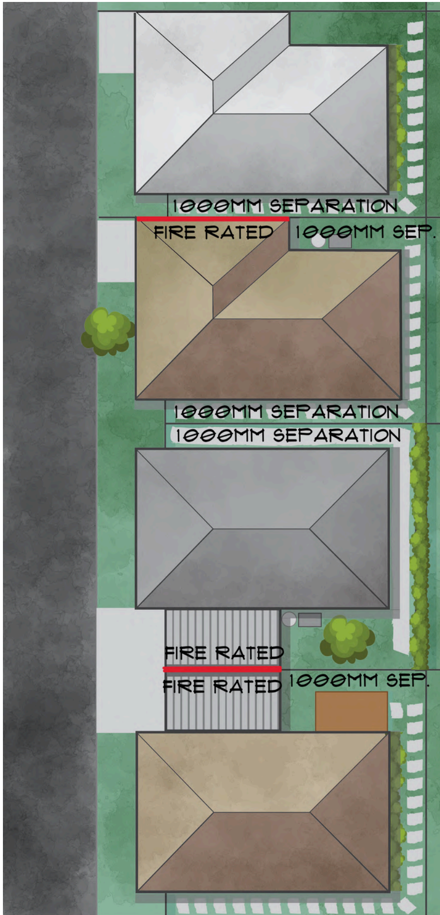
Figure 15: Fire separation between structures.
